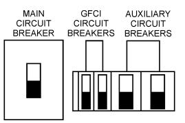
Figure 39. Main, Aux. and GFCI Circuit Breakers (OFF)
